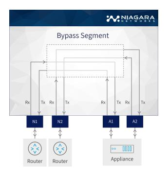
In normal inline mode, the common network deployment for inline security devices such as firewalls and intrusion prevention systems, traffic from one side of the network is forwarded to the inline appliance, and through the inline appliance to the other side of the network.
