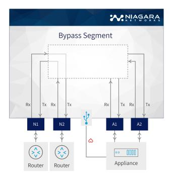
The appliance sends an external heartbeat via the USB port. As long as the heartbeat is received, the segment stays in normal mode and the appliance is inline with the newtwork link.
