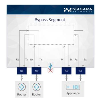
In case an external heartbeat is not received for the appropriate segment, and the count down timer for that segment expires, the affected segment will go into bypass mode.
